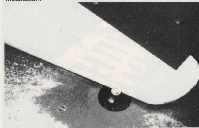
3/16 router bit makes short work of rounding stab leading edges.
