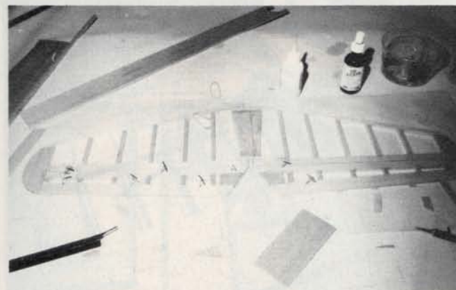
Stab-elevator framed up on Celotex building board.
