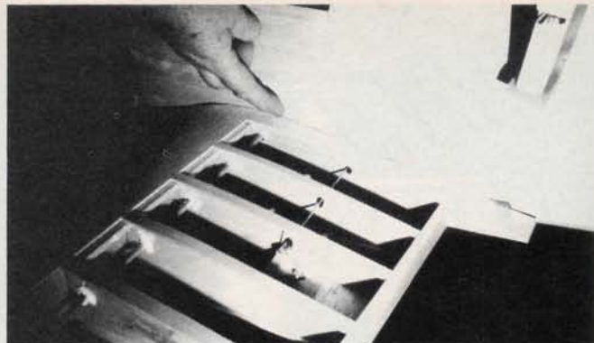
Checking wing-to-fuselage joint. Take your time here — neatness counts.
