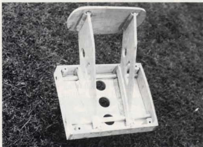
Center section/motor mount prior to 1/32" ply top skinning.
