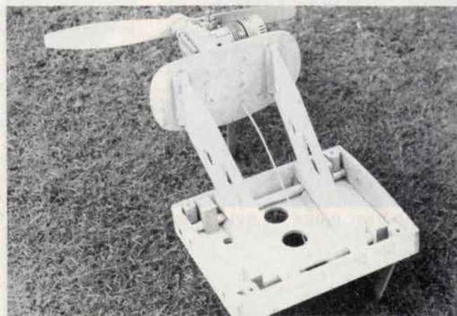
Center section/engine mount; note blocks where wing fixing pins will enter the tubes, also blocks for mounting bolts seen here drilled.
