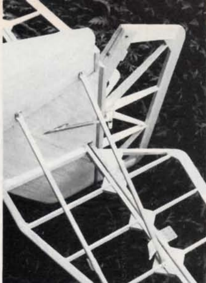
Braced tail unit ensures rigidity at all times.
