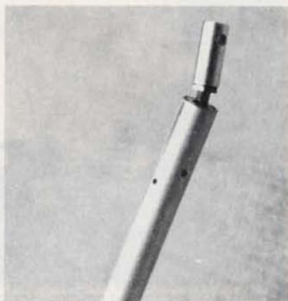
Adjustable top end of rear strut.
