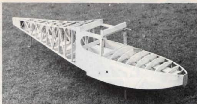
Structure is light and strong, particularly forward of the cabin. 1/32" plywood skin used on hull sides in this area. 1/8" balsa sheet is used to cover top nose section.
