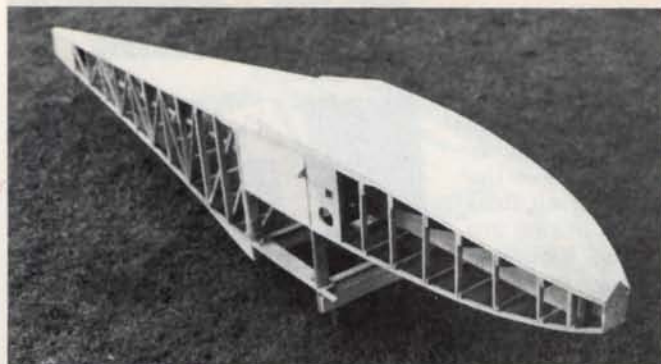
Forward bottom 1/32" ply skins in place, also 3/32" balsa on aft bottom behind step.
