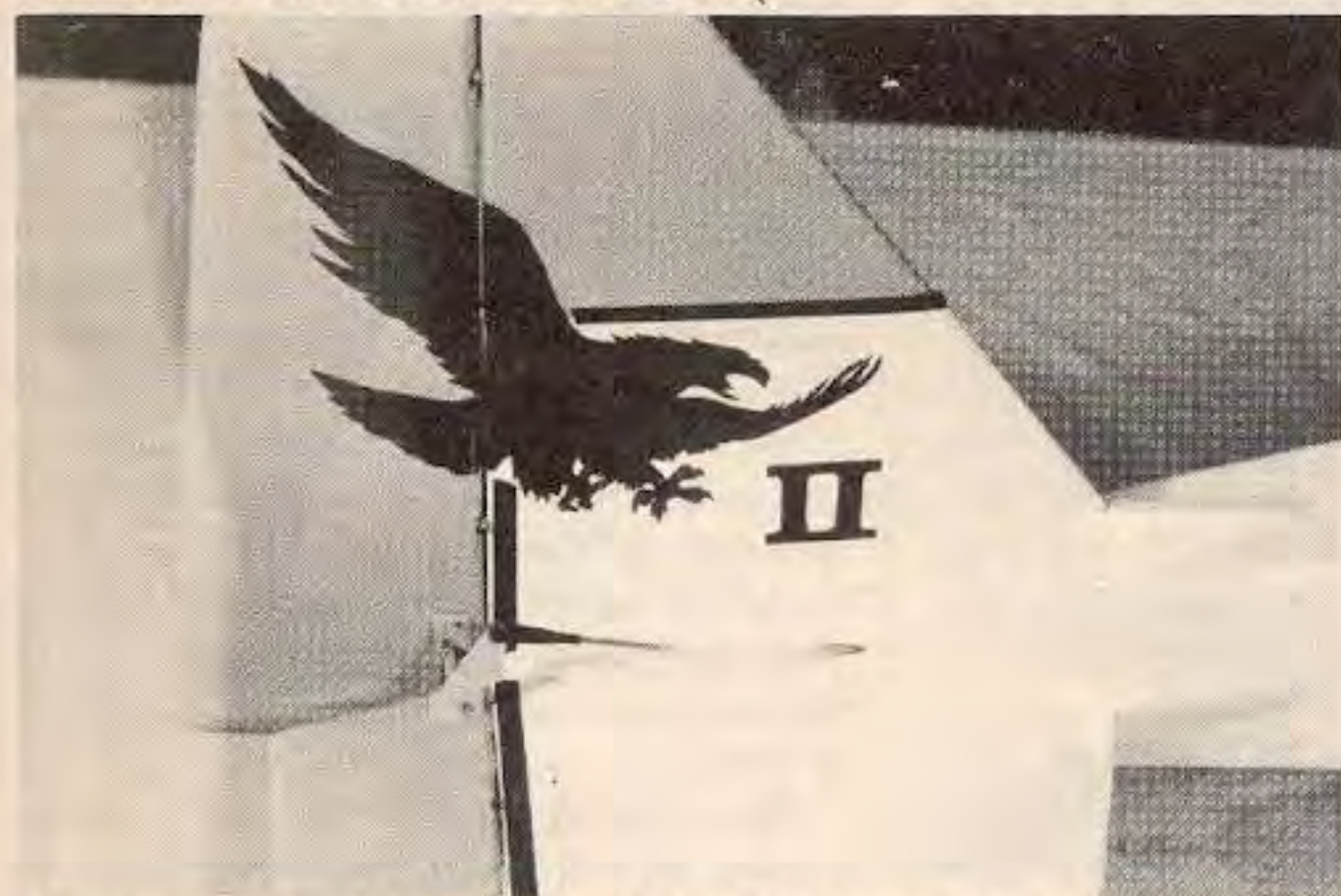
Goldberg control horn and Robart steel pin hinges used. Dorsal fins add nice touch to the tail group. Black MonoKote trim used.
