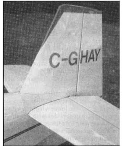
LEFT: Engine exhaust exits through bottom of carburetor intake. Note front strut attachments. MIDDLE: Williams Bros. 1/5th scale pilot busts are glued to the canopy floor with Goop. Elevator and rudder servos extend through floor in rear. RIGHT: 1/64" plywood fin-stab fairings really clean up the tail.
