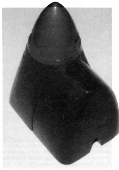
The finished cowl. The upper part is cemented to the engine bulkhead. The lower is easily detached for engine servicing.
