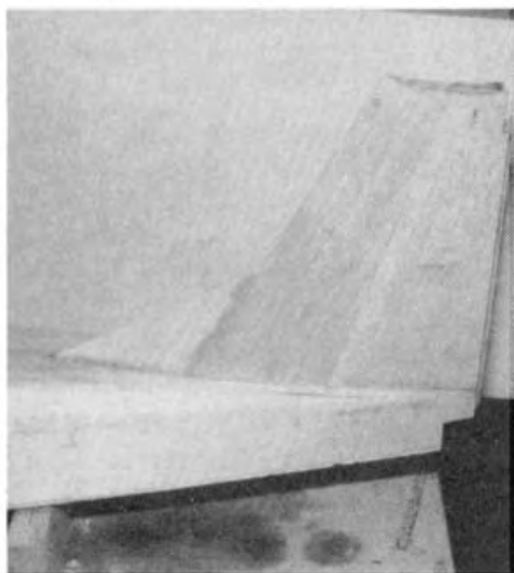
The completed fin. The hull is still in its assembly fixture.
