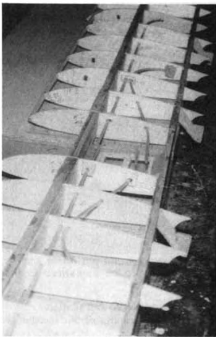
The completed basic wing structure. All ribs and spars are in place, webbs installed and the ply servo mount in the wing center section is installed. Plastic sheaths for flaps and aileron control system have been installed and glued into position. The plastic tubing may be pre-bent to drawing with a heat gun carefully, to avoid melting the plastic.
