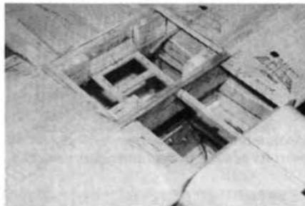
The assembled flap locates the flap support Ribs "B" and "F". Lower spars are in position.
