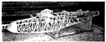
The top cabin block must be supported in position while the cement cures. Then, add the balsa nose block and rear fuselage (turtledeck) formers.
