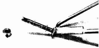
Brass tube is used for the solder Joint instead of soft wire. Very strong. Note flat ground for wheel collar retaining screw.
