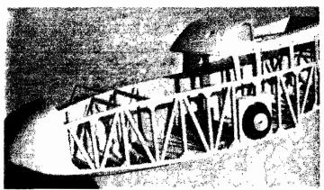
Install cabin floor and landing gear blocks now. Balsa blocks are used as filler for "retracted" wheel location.
