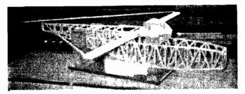
Prior to gluing the top cabin block in place, it must be squared up with the frame to ensure that the wing will be squarely mounted.
