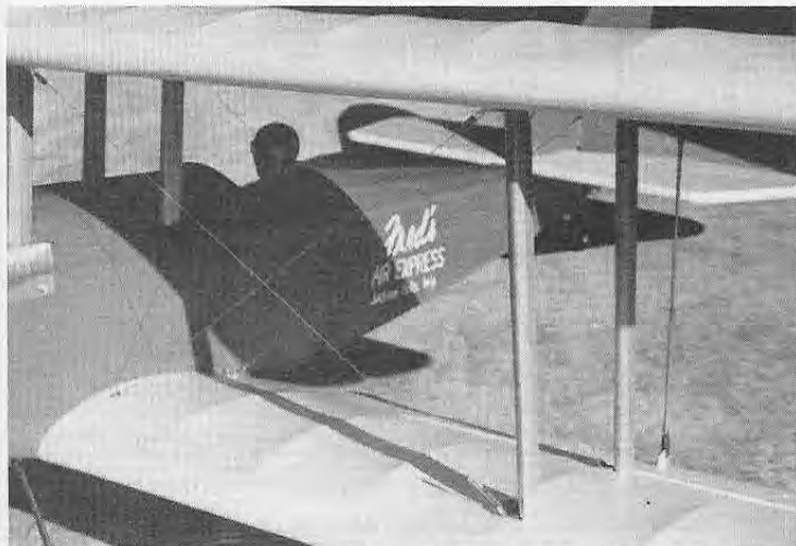
Outboard wing struts and aileron linkage between the wings.
