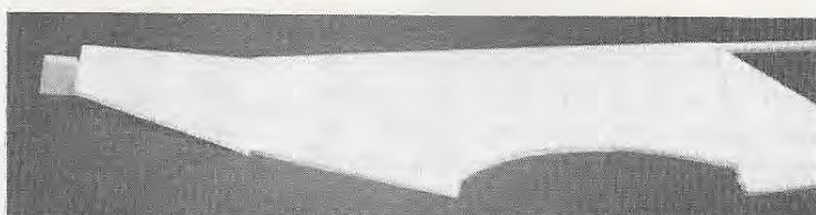
3/16" balsa nose piece is glued to the side, blocked up 3/4".
