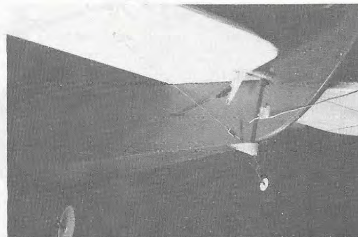
Tailwheel, control horns, pushrods and tail bracing.
