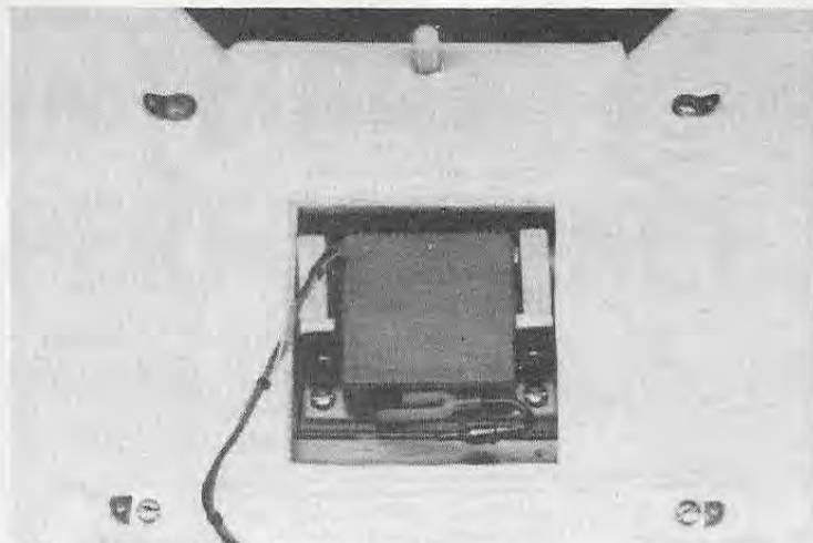
Aileron servo in lower wing.
