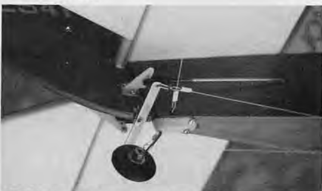
PHOTO 10: Tiller bar on aircraft rudder. Control cables are attached to bent pin hooks with crimped aluminum tube. No need to remove tail wheel.
