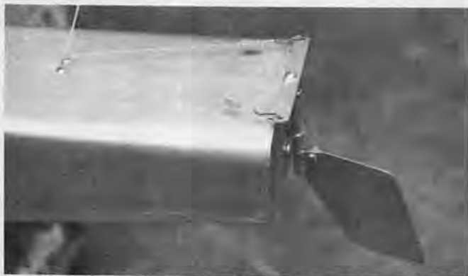
PHOTO 9: Mount steerable rudder to left float. Bent pin hooks allow easy removal of monofilament control cables. Cables run from water rudder through wire "U's" to aircraft rudder.
