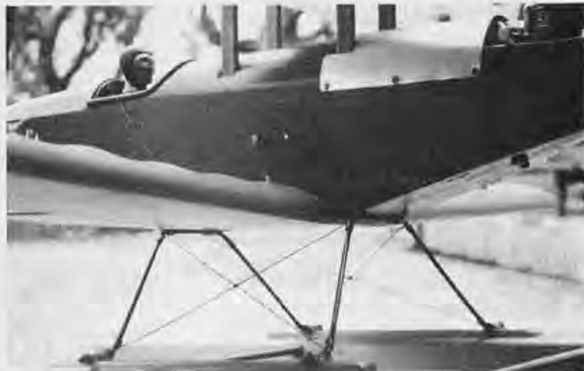
PHOTO 12: 1/16" wire cross braces are soldered to the struts after aligning the floats to the wing.
