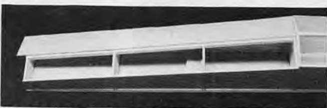
PHOTO 5: Glue on 1/8" sheet balsa bottom.
