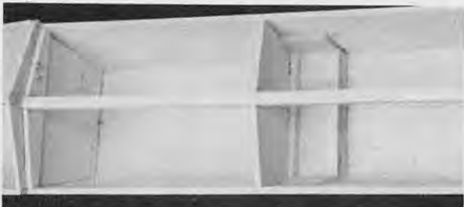
PHOTO 4: Glue in box structures for aluminum spreaders between the two floats.
