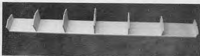
PHOTO 2: Glue bulkheads to 1/4" x 3" balsa top.
