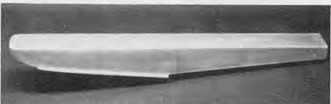
PHOTO 6: Add balsa noseblock and 1/8" plywood transom. Cover floats with 3/4 ounce glass cloth and resin. Glue on 1/4" square balsa spray rail and 1/4" plywood top mounting rail.
