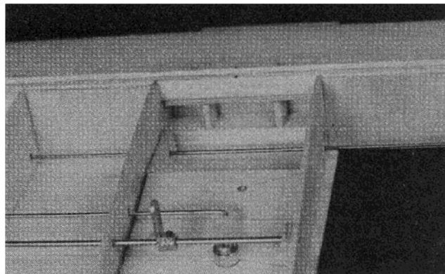
Flap bellcrank and throttle outer torque arm installation. Note blocks between lower spar and ply doubler. These prevent blind nuts from being pushed out.
