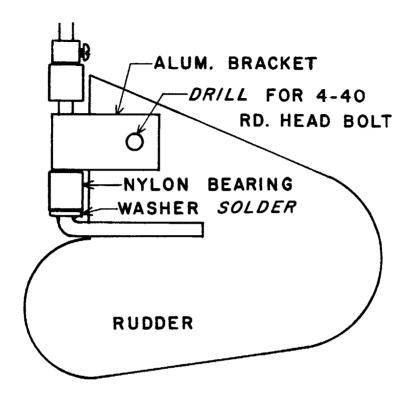
Steerable water rudders take a severe beating--especially on landing. Tests on a special high-powered model brought about this major improvement for much greater strength in the mounting system.
