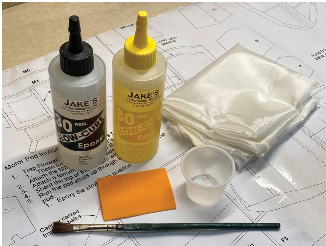
Fiberglassing supplies include resin, fiberglass cloth, a squeegee, brush, and a mixing cup.
