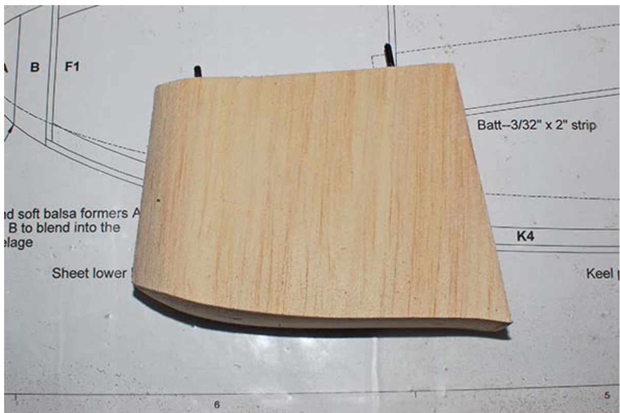
06. After shaping the upper float pad, the pads were joined with 3 mm carbonfiber tubing and the assembly was sheeted.
