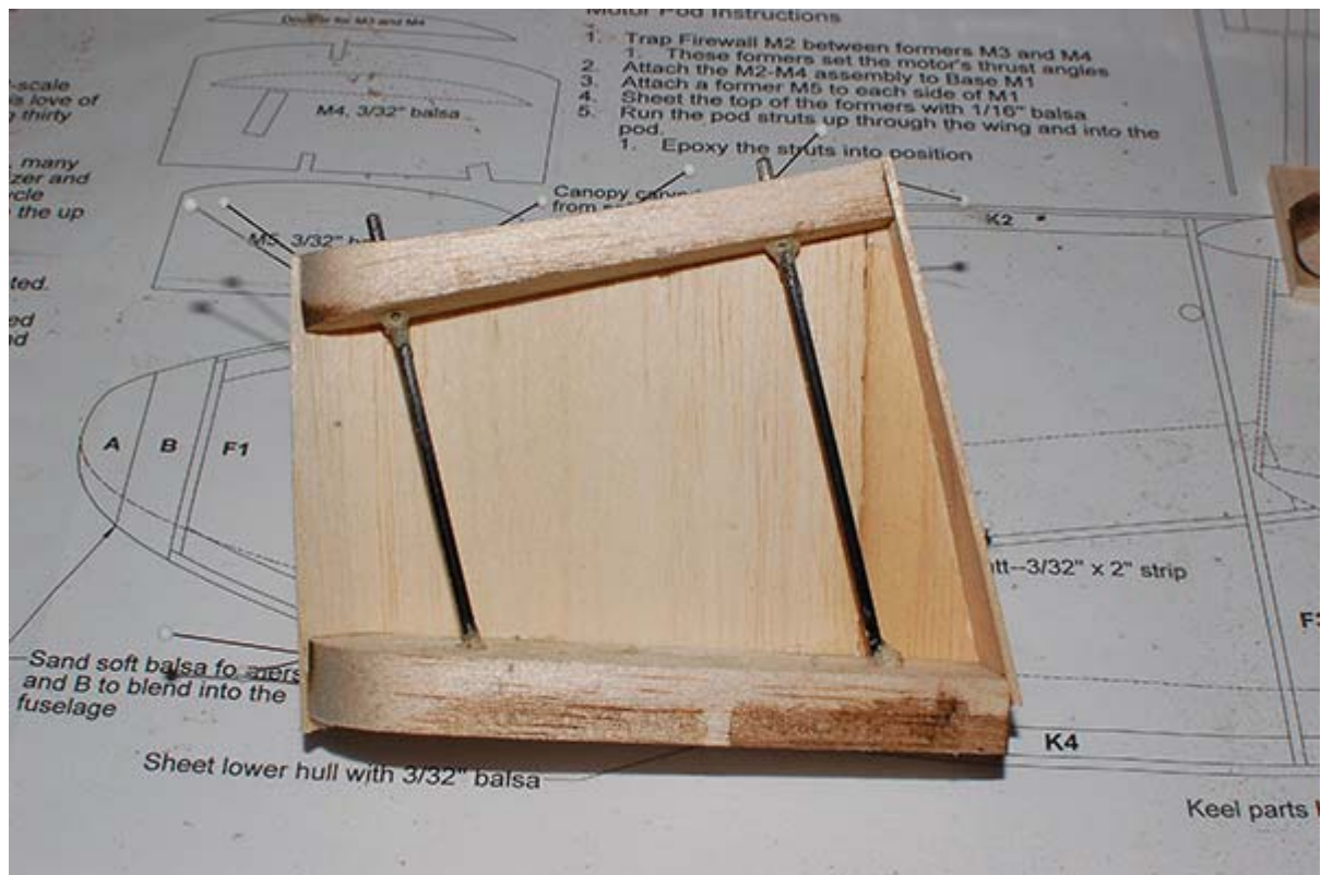
06. After shaping the upper float pad, the pads were joined with 3 mm carbonfiber tubing and the assembly was sheeted.
